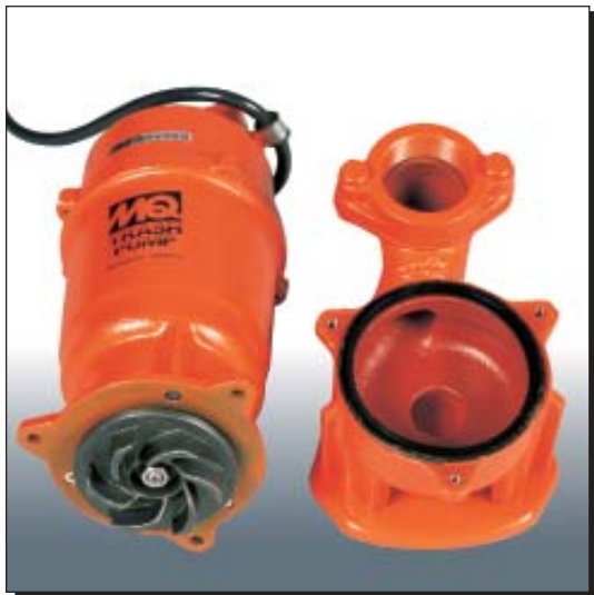
Easy Cleanout — The base of Multiquip Submersible Trash Pumps can be quickly removed for service or inspection.
